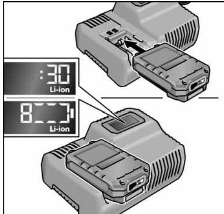
1. Insert the charger mains plug. The display backlighting lights up green for 2 seconds and then goes out again. OK is displayed.
