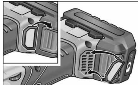
Remove filter cover and blow it out with dry compressed air.
