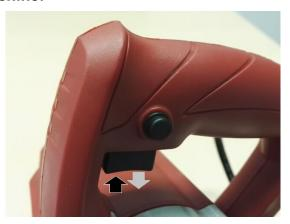
Press and release the trigger switch.
