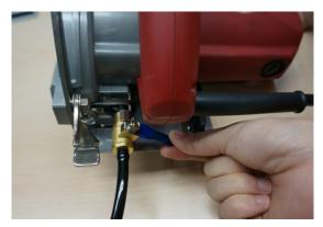
■ Turn the water valve to the position for maximum water flow onto the blade.
