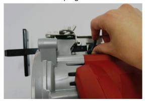
Adjust the parallel guide to the desired width from the blade, then tighten the retaining screw.
