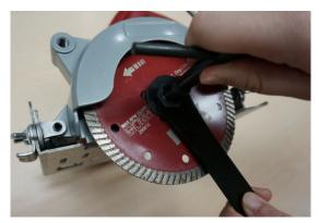
■ Finally, use the socket wrench to tighten the spindle bolt in a counterclockwise direction while using the solid wrench to fix the spindle.
