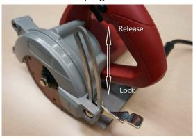
Loosen the cutting depth lever.
